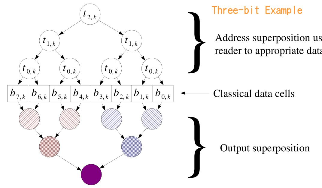
Address superposition used to steer reader to appropriate data cells
