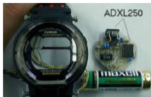
Fig. 1 A photograph of accelerometry device with a built in two ADXL250 acceleration sensor IC chips.
